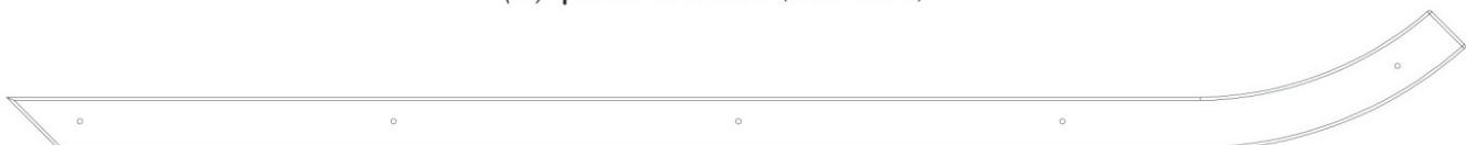
K5 | BORDURE DE TOIT - W4L11678 (x1) | 5/8"x5 1/4"x55" (16x133x1395)
