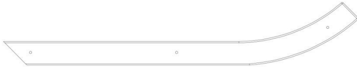
K4 | BORDURE DE TOIT - W4L11795 (x1) | 5/8"x5 1/4"x29 5/8" (16x133x752)
