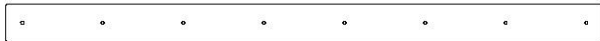
N03 TASSEAU DE TOIT - W4L16172 (x2) 5/8 po x 2 3/8 po x 37 3/8 po (16x60x948)
