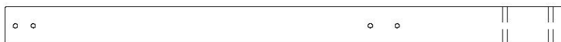
SP71 SUPPORT DE POUTRE DE BALANÇOIRE - W4L16168 (x1) 3 3/8 po x 3 3/8 po x 49 1/2 po (86x86x1256)
