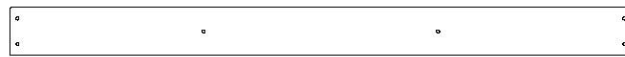
M02 PLANCHE DE PLANCHER - W4L16123 (x2) 5/8 po x 3 po x 38 7/8 po (16x76x988)
