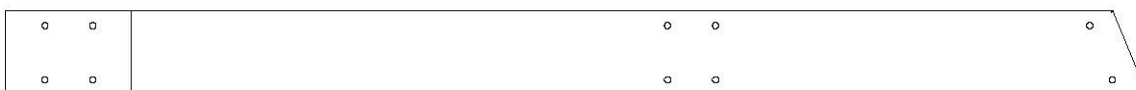
G03 RAIL AU SOL - W4L16132 (x1) 1 po x 5 1/4 po x 71 3/8 po (24x134x1814)
