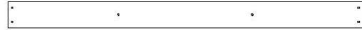
M02 PLANCHE DE PLANCHER - W4L16123 (x2) 5/8 po x 3 po x 38 7/8 po (16x76x988)
