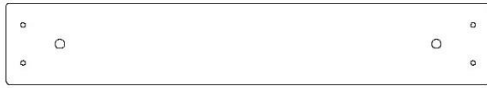
J2 | PLANCHE DE FIXATION - W4L16268 (x1) | 1 po x 3 3/8 po x 20 1/4 po (24x86x514)
