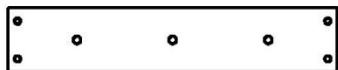
M77 (x1) | CALE DE TOBOGGAN - W100544 5/8 po x 3 3/8 po x 17 1/4 po (16x86x438)
