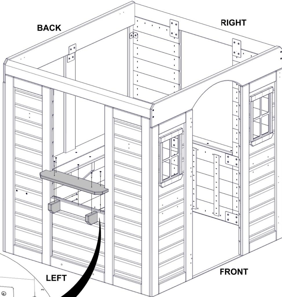
**NOTE: ALIGN SCREWS WITH ALL PILOT HOLES**
