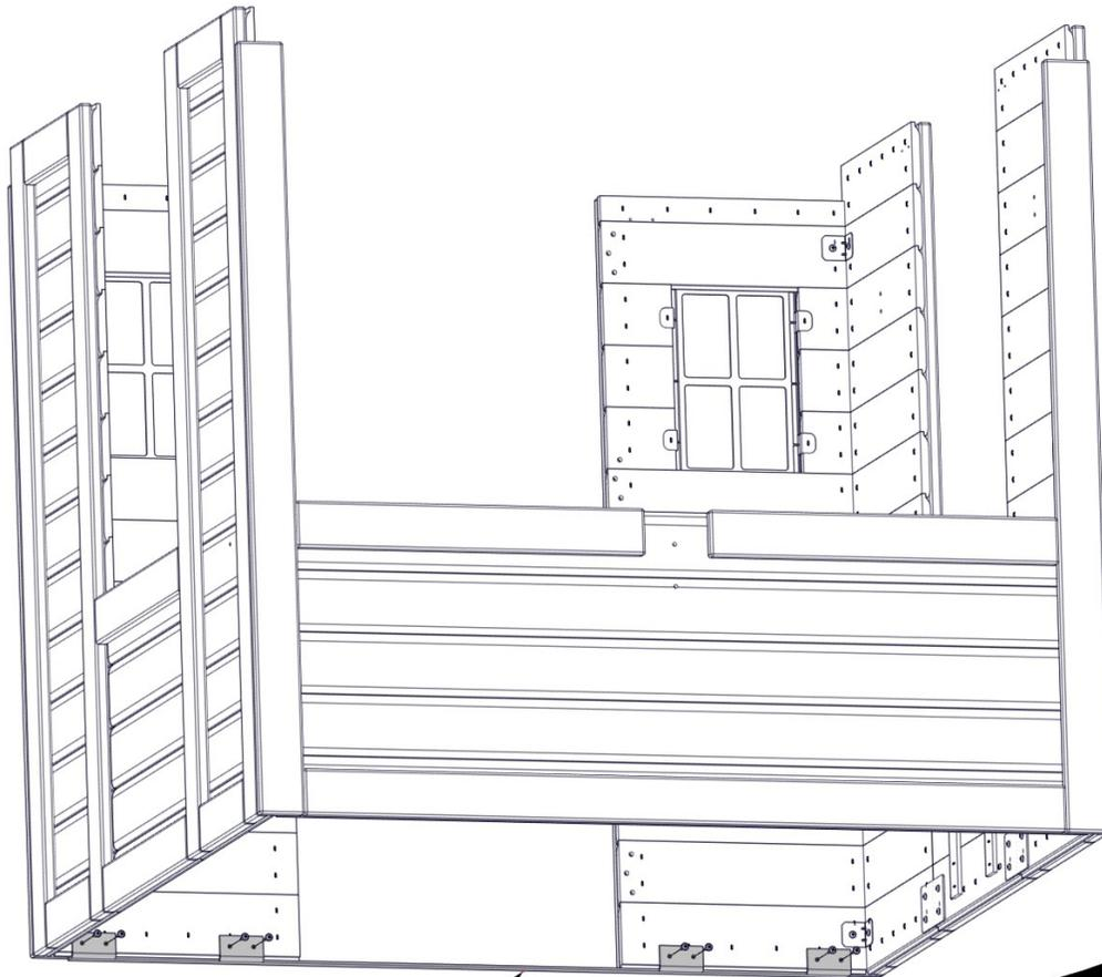
**NOTE: ALIGN METAL TIE STRAP WITH PILOT HOLES IN BOTTOM OF PANELS**
