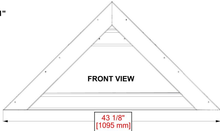
**NOTE: ALIGN K9 BOARDS WITH PILOT HOLES IN GABLE TRIM. FLUSH EDGES**
